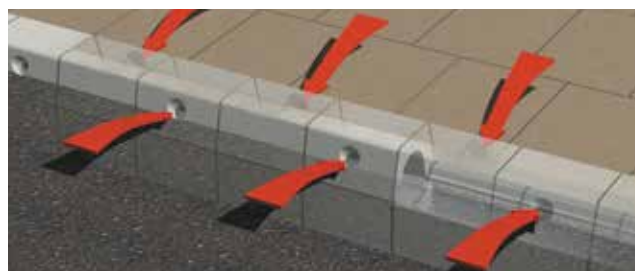
Beany Drainage from both sides using symmetrical top
